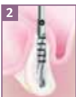
2 SP3D/TSV3DS 3.4/2.8mmD Intermediate Drill
